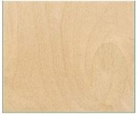
Single piece face has light and uniform colour. A few sound tight knots and pin holes are permitted. Open knots and defects are replaced with small oval or round veneer patches before gluing. The patches are selected to closely match the background colour.
