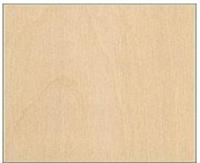
Single piece veneer of light and uniform colour. A few small pin knots and some brown streaks are allowed. Veneer of this grade is intended for natural finishes. Patches are not allowed. The majority of Grade B veneers are the equivalent of the American "white birch" faces.
