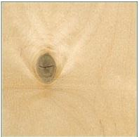
Open defects such as open knots and veneer splits are allowed. Sanding is not required. Recommended for the building of containers and dust panels; can be used for crating and in manufacturing, where construction and strength are more important than the appearance.
